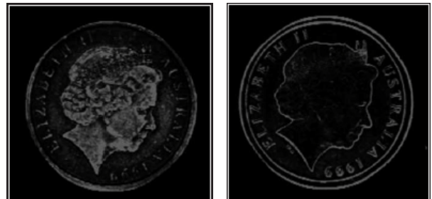
An IDBA-QC360 Bar Light (left) illuminates a coin from above and below (above left) and from left and right (above right).
