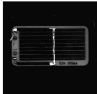
Solar Battery Panel Illuminated by a 150mm (6") Diameter IDD-KH150W
