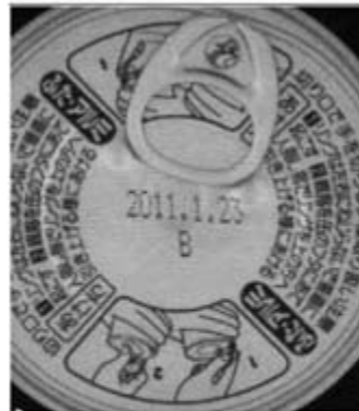
The IFH Thin Type Dome Eliminates Shadows and Reflections on the Shiny and Dimpled Surface of this Pop-Top Can
